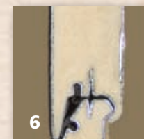
6 Dual acting, between section joint seals
